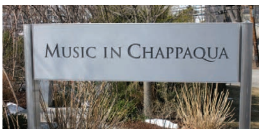
Waterjet-cut 1/8-in. aluminum panels with extrusion frame , mounted on half-round extrusion posts. Lettering is done with perforated translucent film and has internal LED illumination. All the aluminum on the 16-by-60-in. sign was sanded then clear coated.
