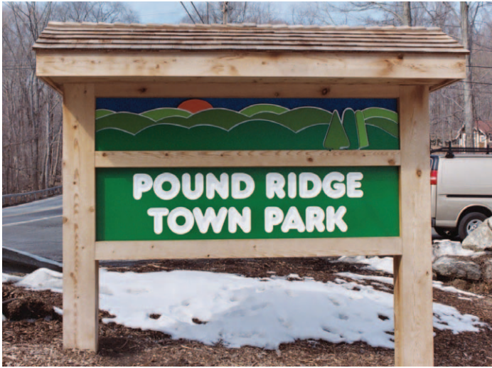
Carved 1½-in. high-density urethane board finished with acrylic Polyurethane paint; landscape graphic is multiple layers of ¾-in. HDU board. Each section is 2 by 8 ft., with a cedar framework, posts and roof.
