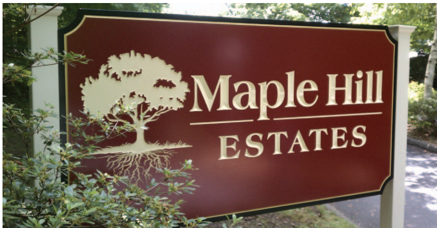
Carved graphics on 3-by-6-ft. panel of 1½-in. HDU, finished with acrylic polyurethane paint and mounted on PVC posts
