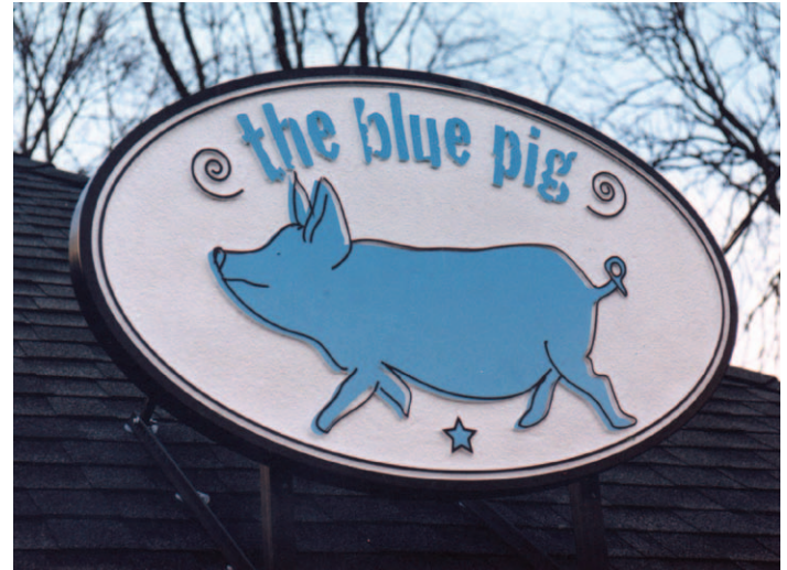
Pebble-blasted 3-by-5-ft. panel of 2-in. HDU board , finished with acrylic polyurethane paint and mounted on custom-made roof brackets
