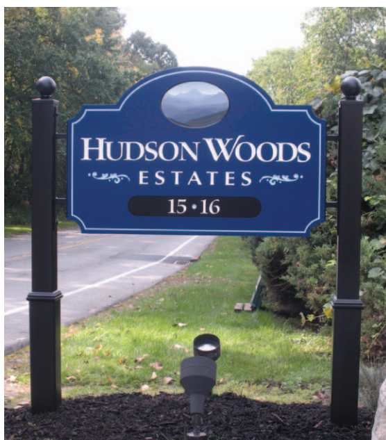
Carved lettering on double-sided 30-by-38-in. panel of Extira, finished with acrylic polyurethane paint. Graphic is a digital print, and sign is mounted on powder-coated, custom-made steel brackets on PVC posts with 4- to 5-in. transition.
