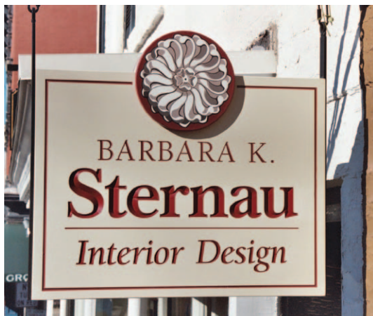
Carved lettering on double-sided 18-by-24-in. panel of 1¼-in. Extira. Graphic is a digital print on 1-in. HDU board.
