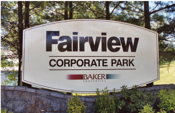
Vinyl graphics and digital print logo on 6-by-15-ft. single-sided aluminum pan-construction sign with aluminum trim
